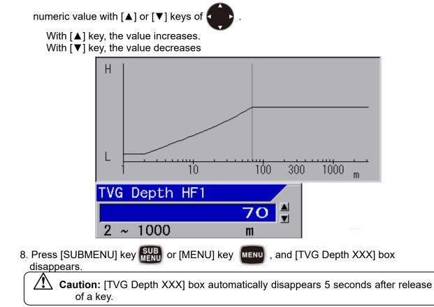
9. In the case of [TVG Adjust High 1], set [TVG Adjust HF1] by increasing or decreasing the
