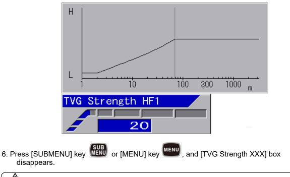
**Caution:** [TVG Strength XXX] box automatically disappears 5 seconds after release of a key.
