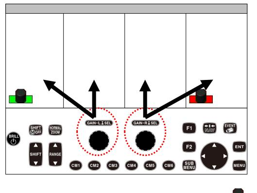
The gain can be adjusted of the screen in which [Gain knob icon] of (red) or (green) is shown at the lower left of screen.
