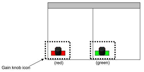
2. To turn [Gain knob icon] to (red), press [GAIN-L/SEL] for the left screen and [GAIN-R/SEL] for the right screen until [Gain knob icon] turns (red).
