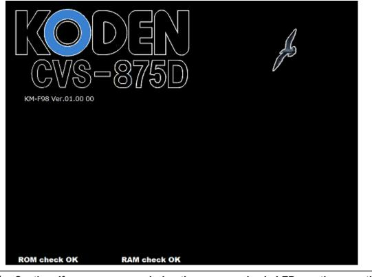
Caution: If an error occurs during the memory check, LEDs on the operation panel blink to indicate possible failure of the unit. In this case, please contact a dealer of Koden or Koden.
