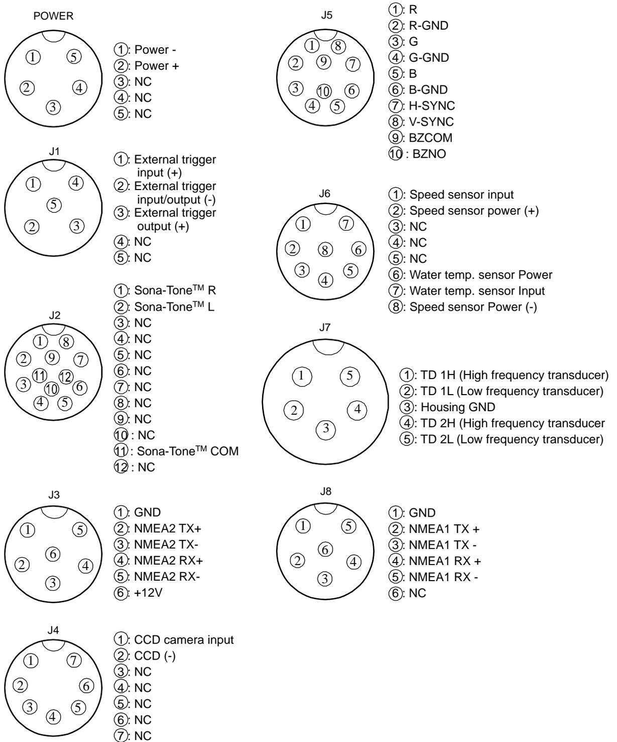
**Fig. 1.20 Pins assignment of rear connector-1**
