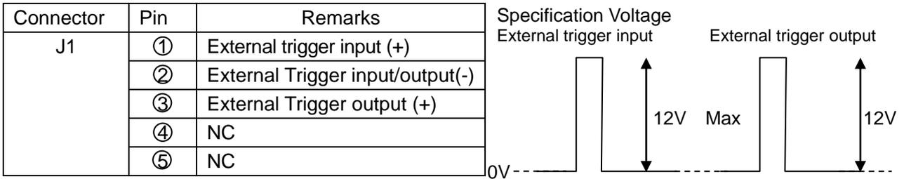
**Fig. 1.27 External trigger**
