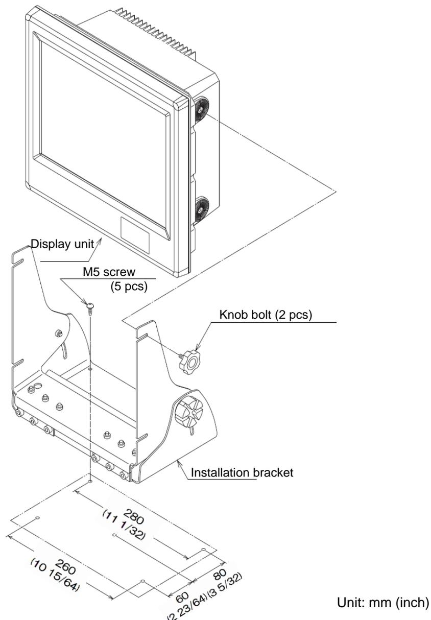
**Fig. 1.2 Desk-top installation of Display unit**
