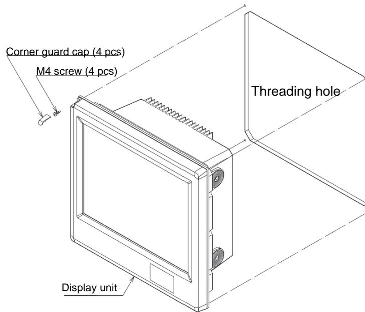
**Fig. 1.4 Flush-mount installation**
