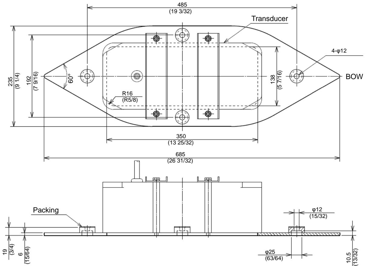
**Fig. 1.12 Outline view of a Transducer unit on steel boat**
