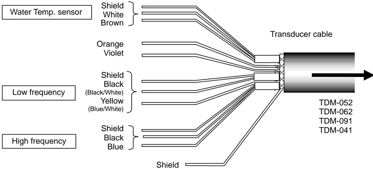
Fig. 1.25 Details of transducer cable
