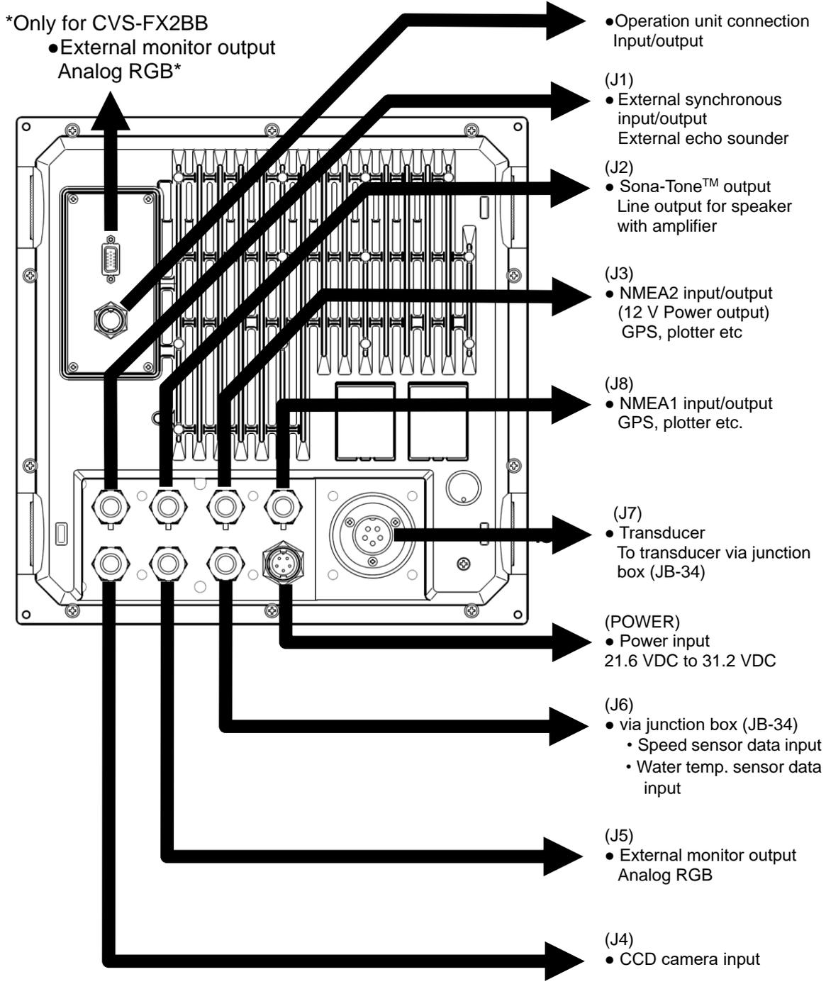
**Pin assignment of rear connectors**
