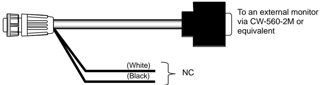
Fig. 1.29 Connection of External Monitor-1
