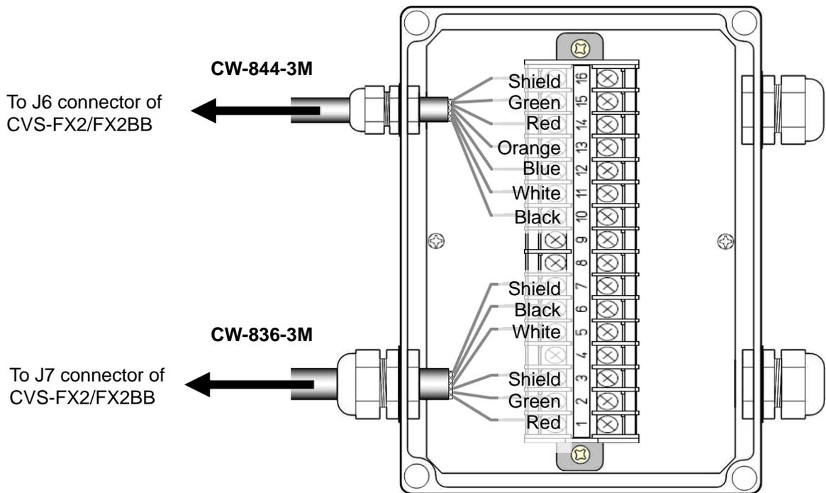
**Fig. 1.24 Connection between CVS-FX2/FX2BB and junction box**
