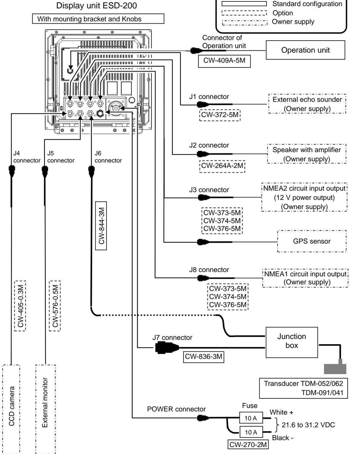
Connection diagram of CVS-FX2BB
