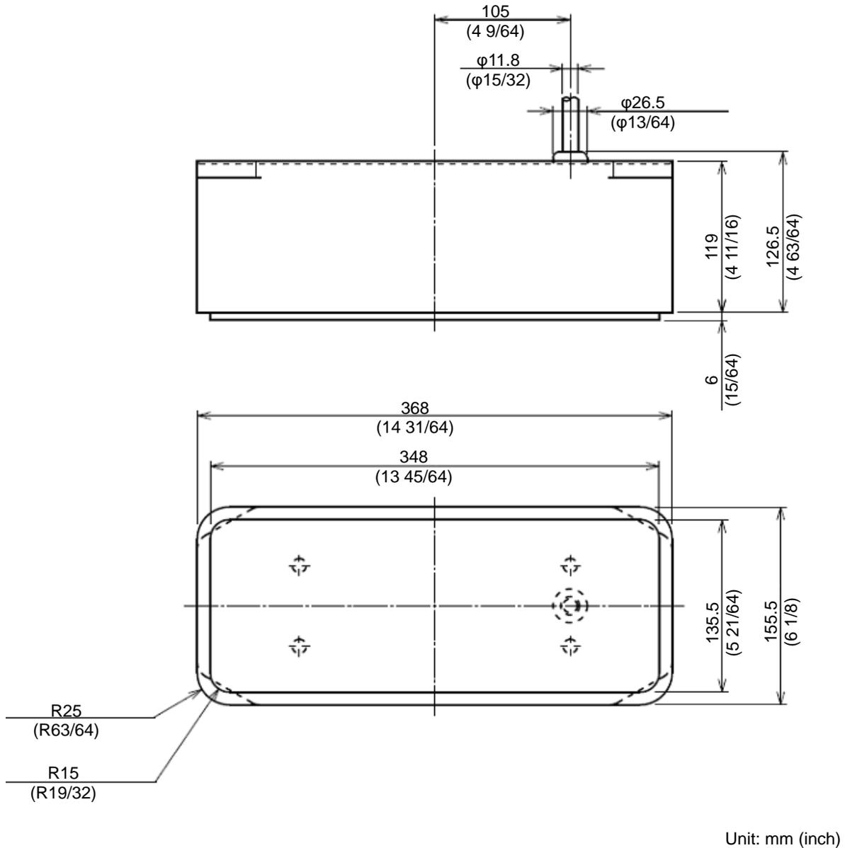
**Fig. 1.17 Outline dimensions of a transducer (TDM-052 and TDM-062)**
