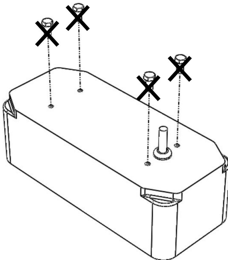
Fig. 1.18 Caution concerning equipment of transducer (TDM-052, TDM-062)
