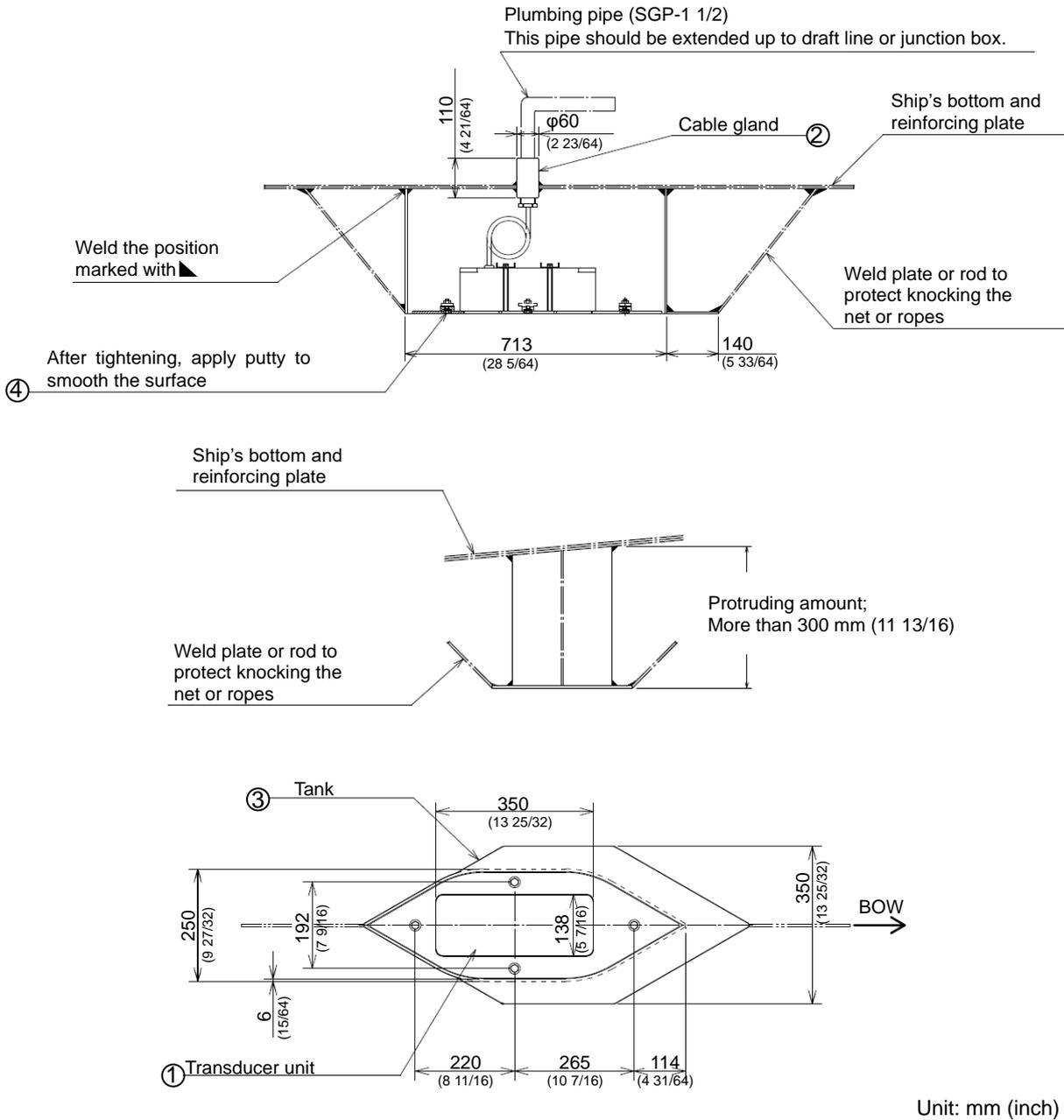
Fig. 1.11 Mounting of a transducer on steel boat
