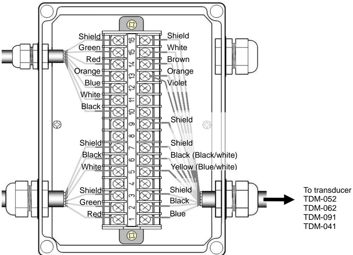
Fig. 1.26 Connection between junction box and transducer
