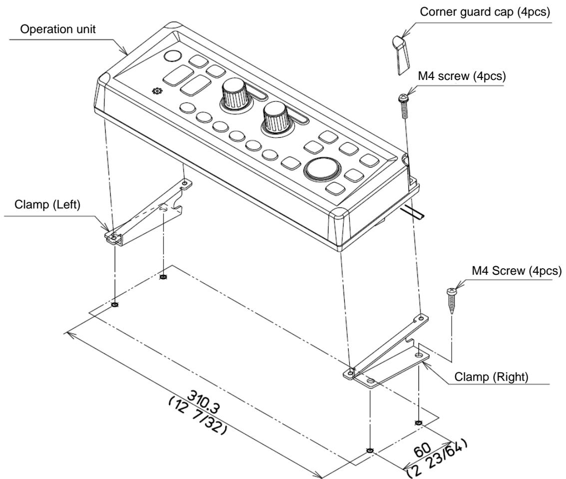
Fig. 1.7 Desk-top installation of Operation unit
