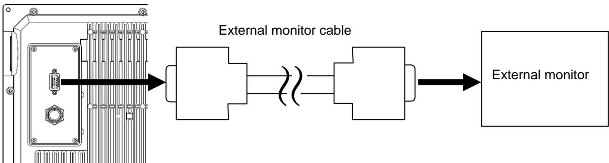
Fig. 1.30 Connection of External Monitor-2
