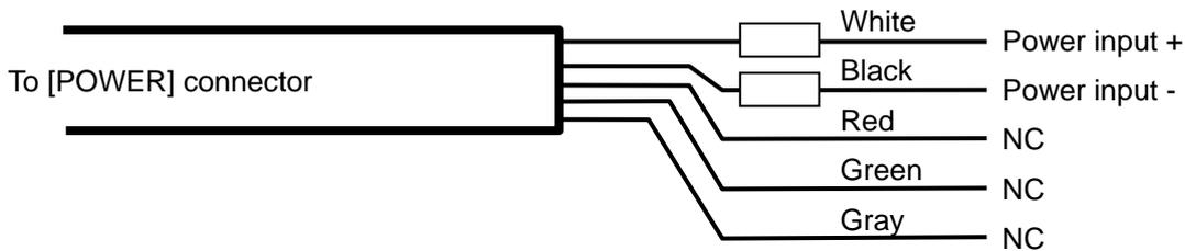
Fig. 1.22 Connection of DC power cable
