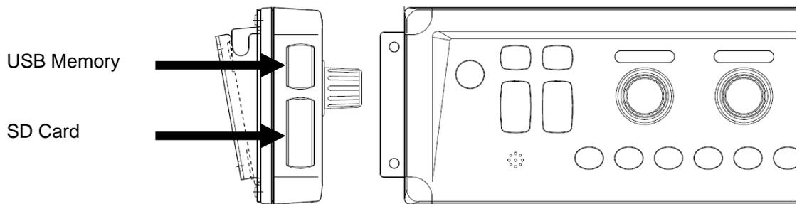
**Fig.1.32 Connection of USB Memory and SD Card**
