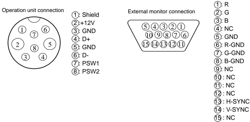
Fig. 1.21 Pins assignment of rear connector-2
