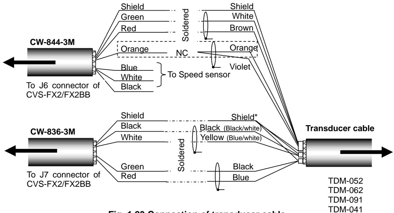
**Fig. 1.23 Connection of transducer cable**
