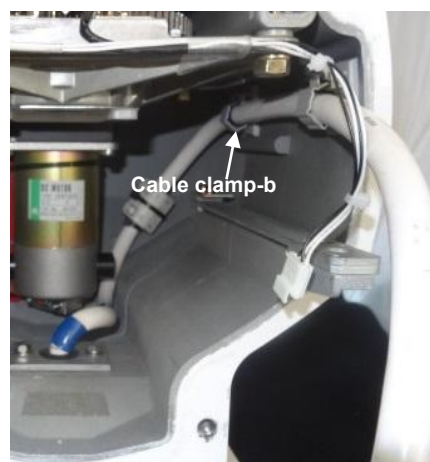
14) Clamp the cable by the cable clamp-b.
