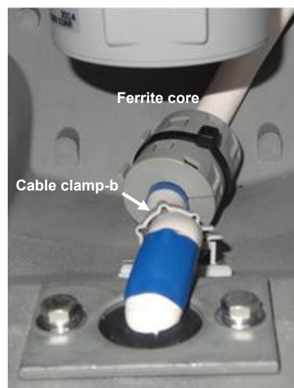
14) Clamp the cable by the cable clamp-b.
