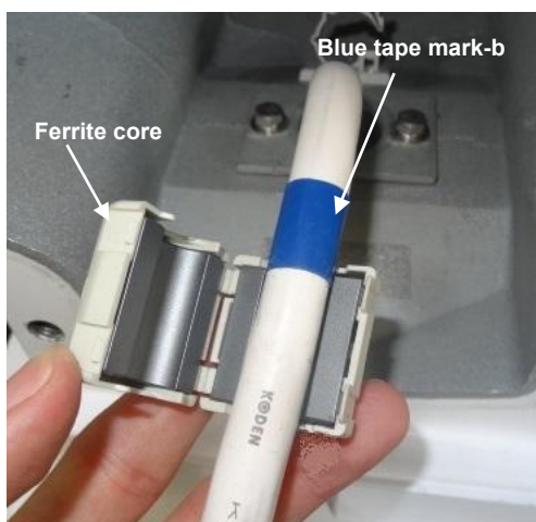
11) Attach the ferrite core to side of the blue tape mark-b.
