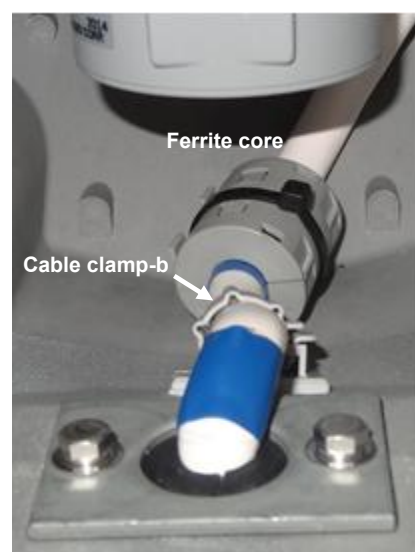
14) Clamp the cable by the cable clamp-b.
