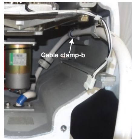
14) Clamp the cable by the cable clamp-b.
