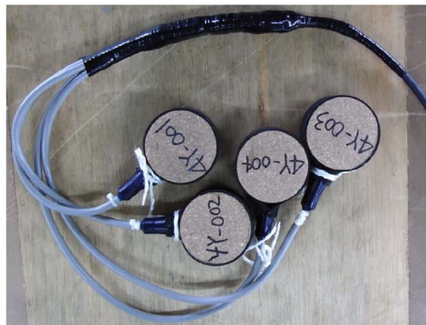
図16.防水処理(参考)完成/FIG 16. Waterproof treatment (reference) completed
