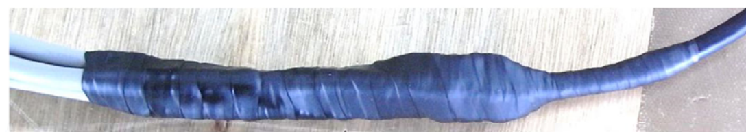
図14.防水処理(参考)/FIG 14. Waterproof treatment (reference)
