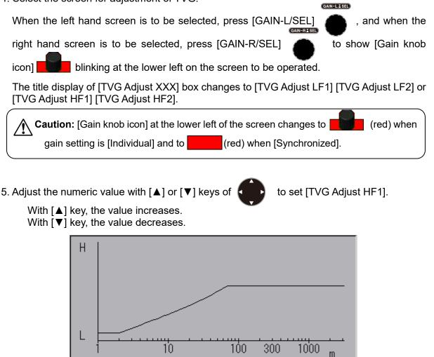
6. Press [SUBMENU] key with or [MENU] key with and [TVG Adjust XXX] box disappears.
