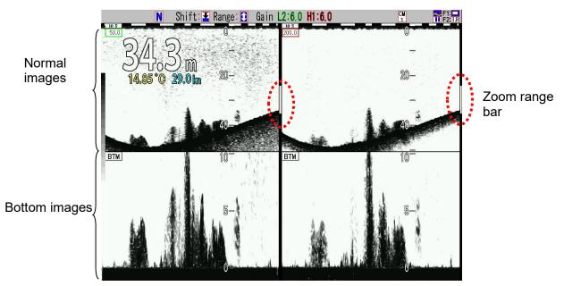
Sea bottom is fixed at 10 to 50% bottom of the screen, and the image above is displayed in the specified zoom range. As the image on sea bottom is magnified, this is an effective zooming mode to identify fish schools, etc. near the bottom.
