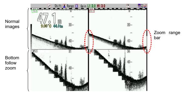
In a specified zoom range, the sea bottom is displayed by automatic shift to be displayed within a range between 30 % and 90 % from the top of images.
