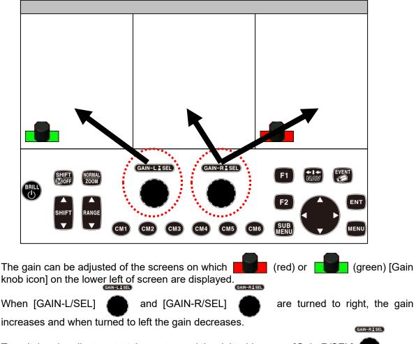
To switch gain adjustment at the center and the right side, press [Gain-R/SEL]
