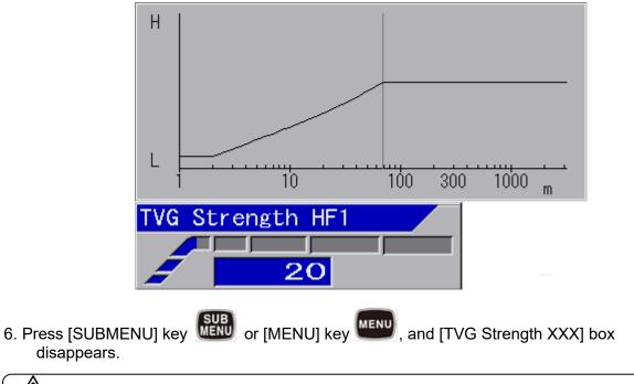
∆ Caution: [TVG Strength XXX] box automatically disappears 5 seconds after release of a key. 7. In the case of [TVG Depth HF1], set [TVG Depth HF1] by increasing or decreasing the
