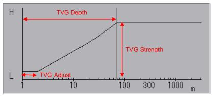
[TVG Depth] determines the depth reference point of TVG correction.
