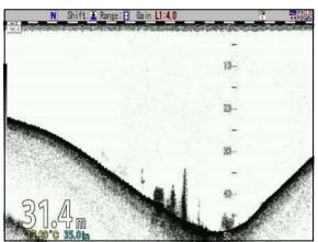
Image after rejection of interference
