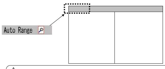
**Caution:** During the operation of auto range, [Range] and [Shift] keys are disabled. In addition, the range operation is set to [All Screen Same], and the [Scr. Individual] range and the [Scr. Individual] shift are not available either.
