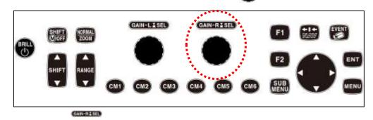
If [GAIN-R/SEL] is turned to right, the gain increases, and the gain decreases if turned to left. The gain knob at the left side is invalid.
