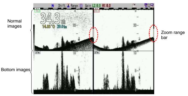
Sea bottom is fixed at 10 to 50% bottom of the screen, and the image above is displayed in the specified zoom range. As the image on sea bottom is magnified, this is an effective zooming mode to identify fish schools, etc. near the bottom.
