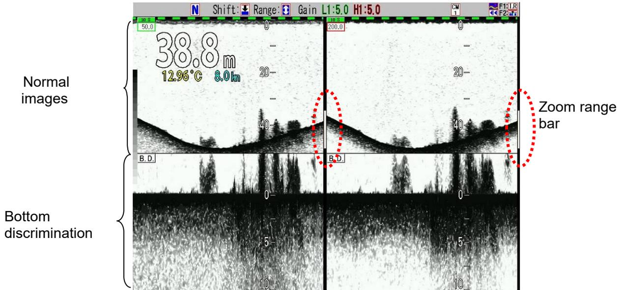
Sea bottom is fixed at 10 to 50% bottom of the screen, and the image of bottom is displayed in the specified zoom range.
