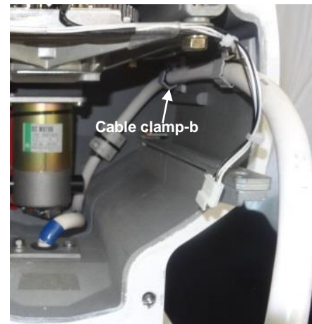
14) Clamp the cable by the cable clamp-b.
