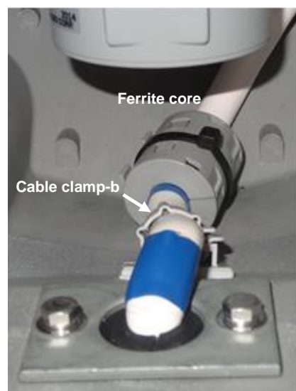
14) Clamp the cable by the cable clamp-b.
