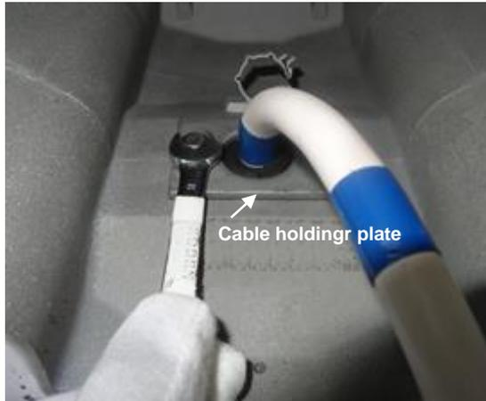
10) Attach cable holding plate and fix it with two bolts.
