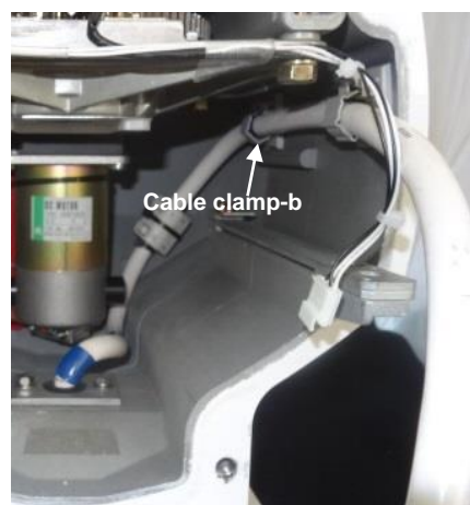
14) Clamp the cable by the cable clamp-b.
