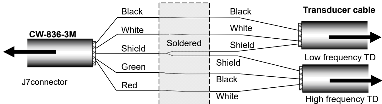
Fig. 5.6.2 CW-836-3M transducer connection diagram
