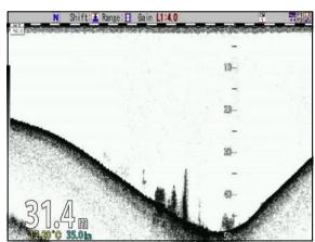
Image after rejection of interference
