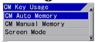
7. Press [MENU] key MENU, and the SUBMENU disappears and the CM key is set to [Setup one touch switching].
