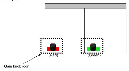
2. To switch over [Gain knob icon] to (red), keep pressing [GAIN-L/SEL]
