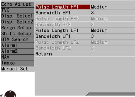
[Pulse Length HF1] of the menu is displayed. Move the cursor with [▲] or [▼] keys of , and select one of [Short], [Medium] or [Long].
