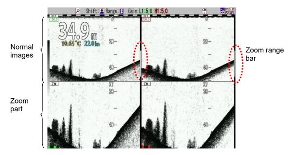
Specifying a shift position, the image under the position is displayed in the specified zoom range.
