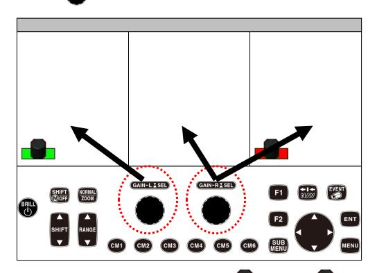
The gain can be adjusted of the screens on which knob icon] on the lower left of screen are displayed.
