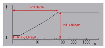
[TVG Depth] determines the depth reference point of TVG correction.
