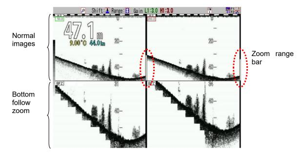
In a specified zoom range, the sea bottom is displayed by automatic shift to be displayed within a range between 30 % and 90 % from the top of images.
