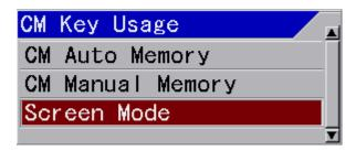
7. Press [MENU] key MENU, the SUBMENU disappears and CM key is set at [Screen Mode Switching].
