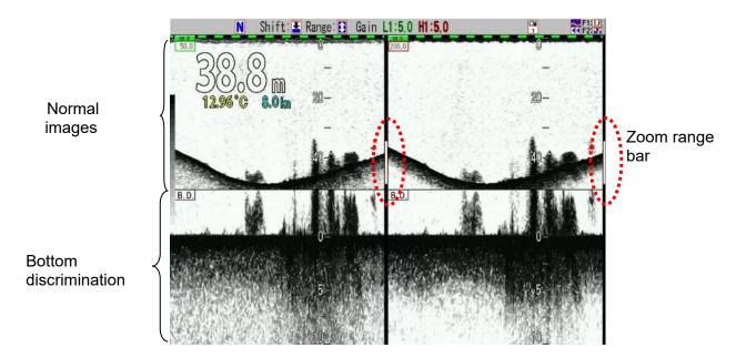
Sea bottom is fixed at 10 to 50% bottom of the screen, and the image of bottom is displayed in the specified zoom range.
