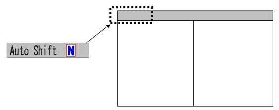
Caution: During the operation of auto shift, [Shift] key is disabled. In addition, the shift operation is set to [All Screen Same], and the [Scr. Individual] range and the [Scr. Individual] shift are not available either.
