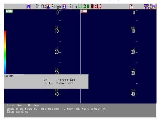
Press and hold the [BRILLO] key to turn off the power to check the TD connection.
