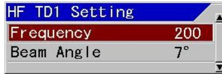
4. Select [Frequency] for changing of frequency, and [Beam angle] for changing of beam angle with [▲] and [▼] keys.
