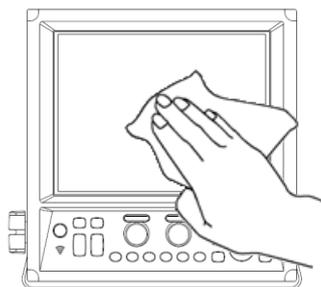
For cleaning the chassis, do not use solvent such as thinner or alcohol. Painting on the surface and characters at the operating unit may be dissolved. After wiping with soft and clean cloth dipped with diluted neutral detergent, wipe away with dry soft and clean cloth.
