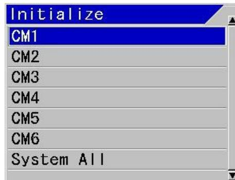
4. When a specified CM is to be initialized, select [CM1] to [CM6] with [▲] and [▼] keys. To initialize the whole system, select [System ALL].
