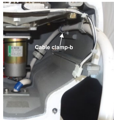
14) Clamp the cable by the cable clamp-b.
