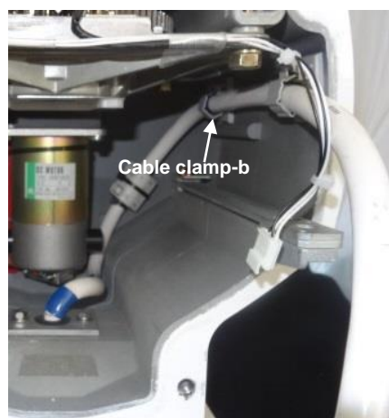
14) Clamp the cable by the cable clamp-b.
