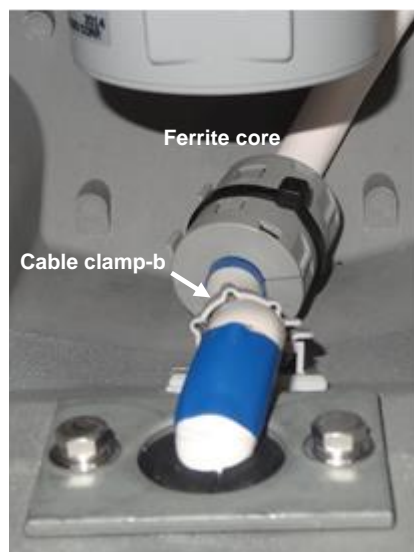
14) Clamp the cable by the cable clamp-b.
