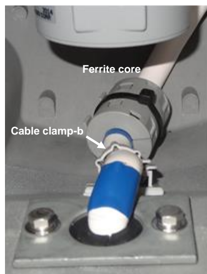
14) Clamp the cable by the cable clamp-b.
