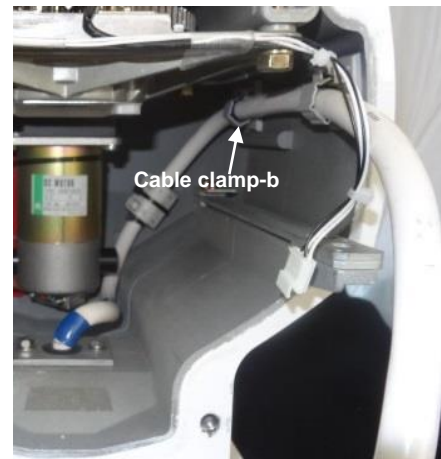
14) Clamp the cable by the cable clamp-b.
